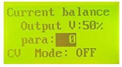
Due to the two sets of secondary output of the transformer, that is, the star or angle connection is connected to the twelve pulse wave control, the current imbalance phenomenon will occur. At this time, the user needs to enter the current balance manually adjust mode.
