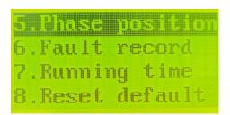
After short pressing the SET button in standby mode, it will remind you to enter the password: ----- (factory password:  $\triangle \triangle \triangle \nabla \nabla \nabla$ ). Press the SET again after entering the correct password to enter the first level menu, the interface is as below.
